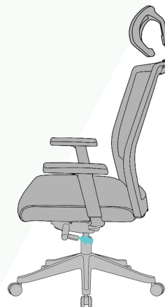
Adjust the handle up and down to lock or unlock the back angle.
